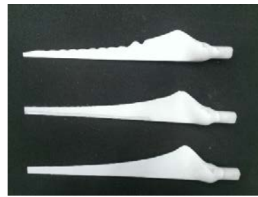
b. (top) tubercle blade (Middle) slotted blade (Bottom) straight blade
