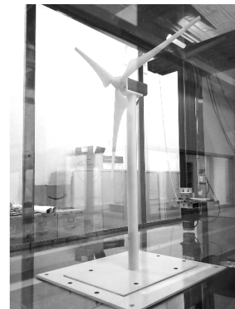
b. Wind turbine blade mounted on motor and column
